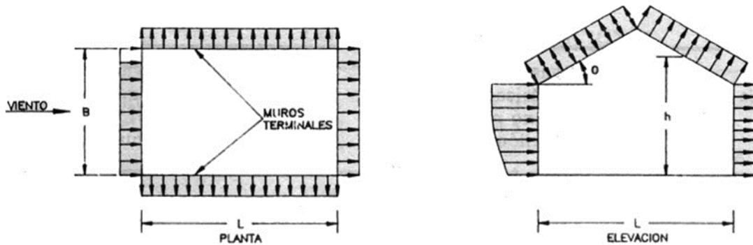
COEFICIENTES DE PRESION EXTERNA PARA MUROS ( $C_p$ )
